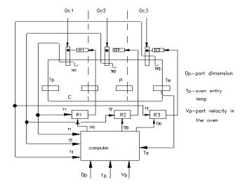
transducers TR1,...,TR4 register the temperature in various points in the kiln and the temperature Te. Computer calculates according to the progress the provided values T10,T20,T30 of the temperature in various points (area) of the kiln. R1, R2, R3 (which include a comparison element) by commanding the execution elements EE1, EE2, EE3 identify the flows Qc1, Qc2, Qc3 to obtain the equality of T1, Y2, T3 with the provided values T10, T20, T30.
